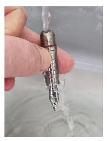
In case the writing block is very dirty, you can immerse it completely safely in a container containing water. Change the water regularly until it remains clear.
